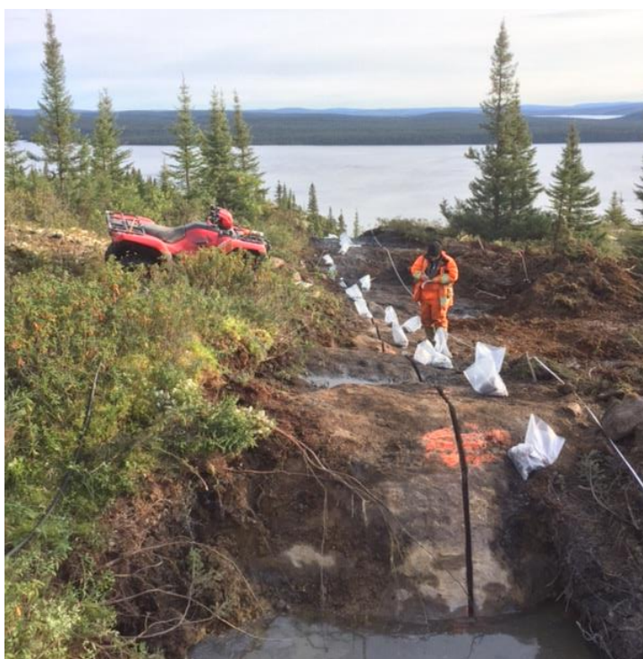
Image 2: Channel sampling being undertaken at the Lac Rainy Graphite Project, Quebec
