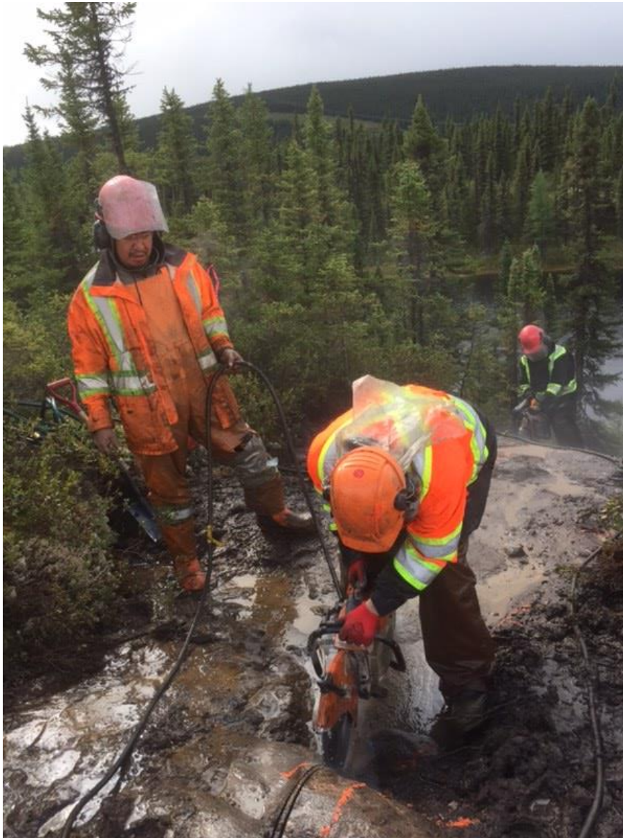
Image 3: Channel sampling being undertaken at the Lac Rainy Graphite Project, Quebec
