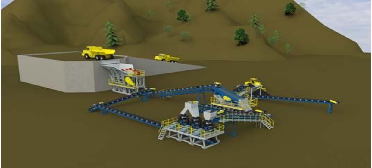
Diagram 7: Sepro Systems 75 tph three stage crushing circuit.
