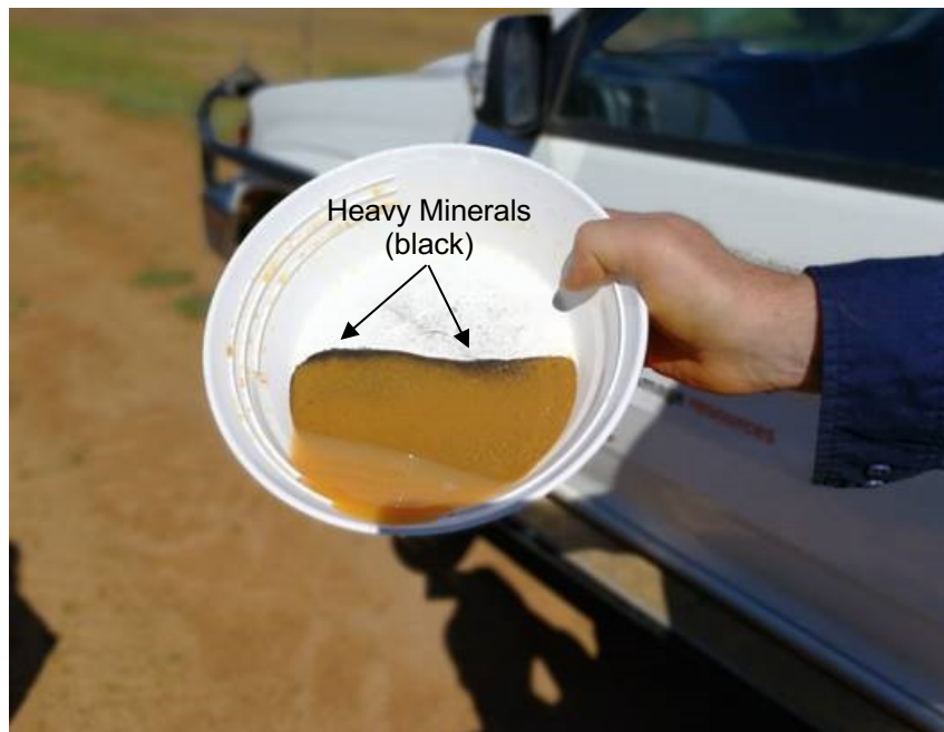
Photo 5: Panning to confirm Heavy Mineral content of ore
