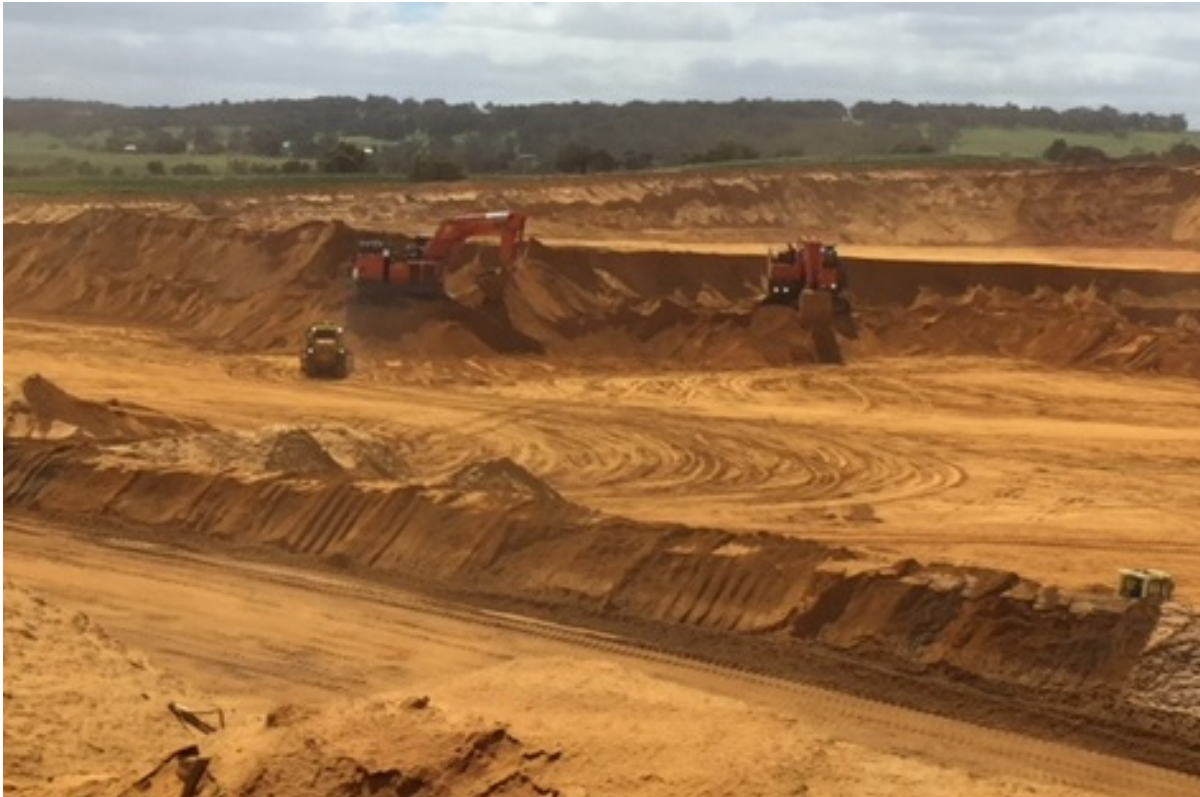
Photo 4: Overburden Removal with Hitachi 3600 Excavators
