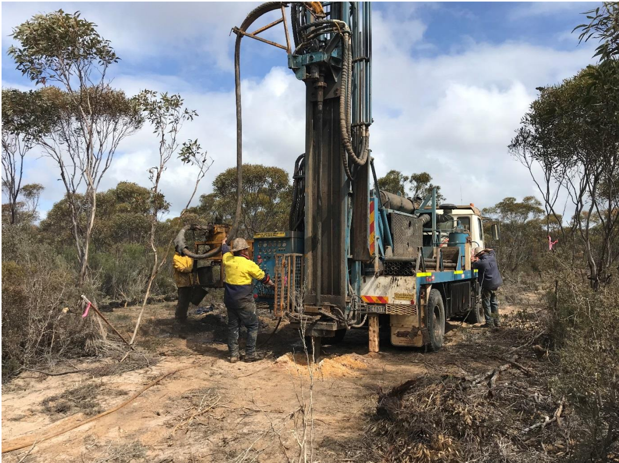
Image 1. Challenge Drilling AC rig in action at Mount Ridley’s auger gold geochemical anomaly drilling program
