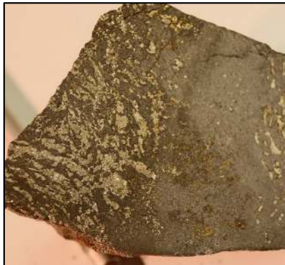
Massive bladed magnetite-pyrite-chalcopyrite skarn
