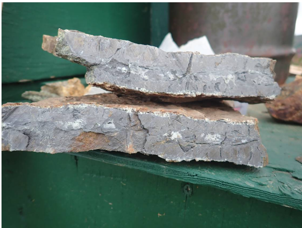
Figure 2. Sample of massive arsenopyrite vein (LQR016, 7.68g/t Au, 30.7g/t Ag).
