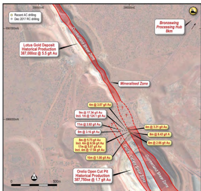
Figure 3: Plan view of Lotus-Orelia with interpreted shear zones.
