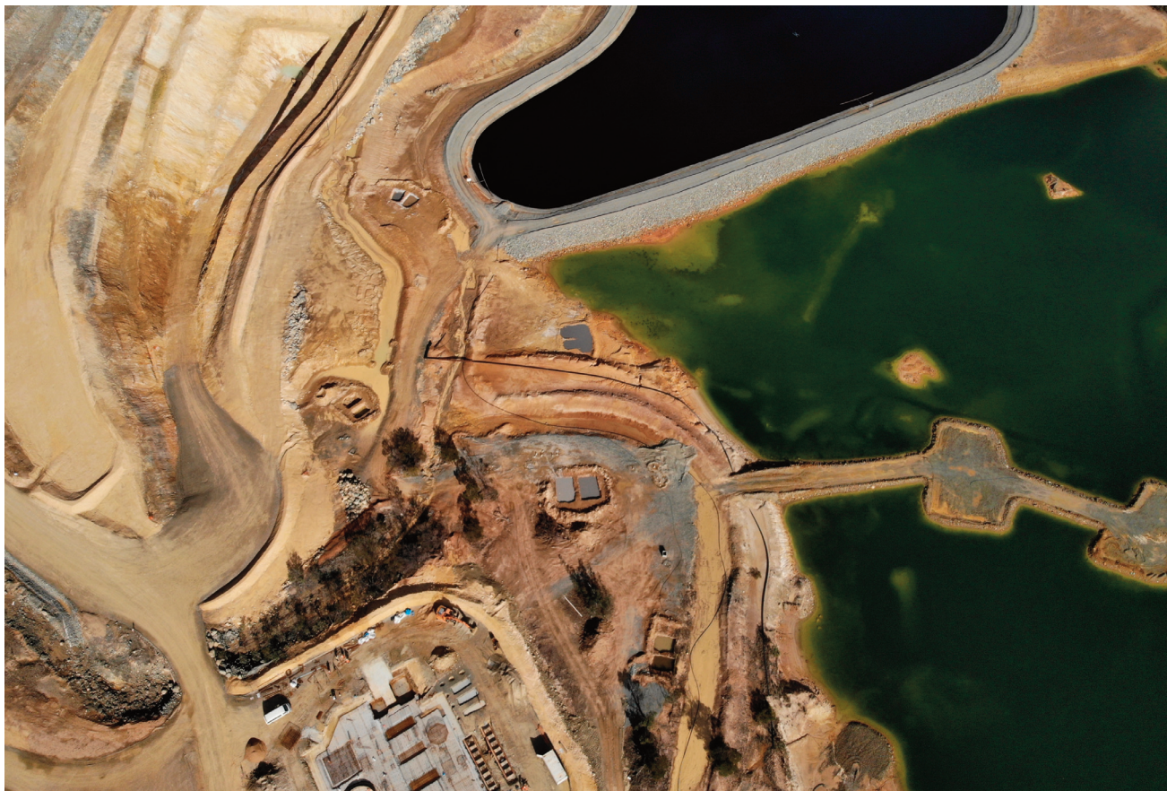
Figure 8: Completed box cut and foundations for the paste plant
