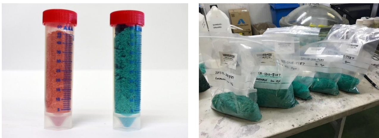
Figure 3: Cobalt and nickel sulphate samples produced from Australian Mines' demonstration plant in Perth.
