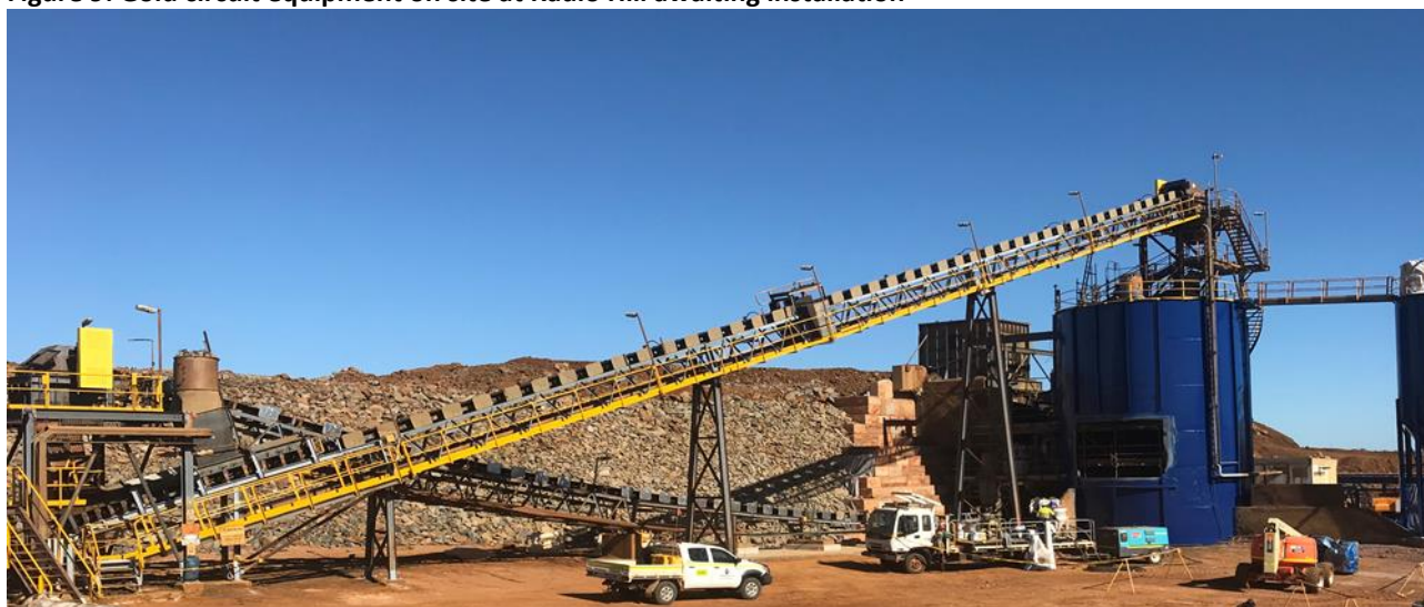
Figure 10: Refurbished crushing circuit and fine ore bin
