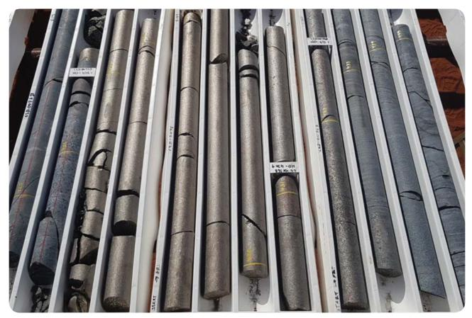
FIGURE 7. Massive sulphide mineralisation (golden coloured core) from upper zone, CZD0076B.
