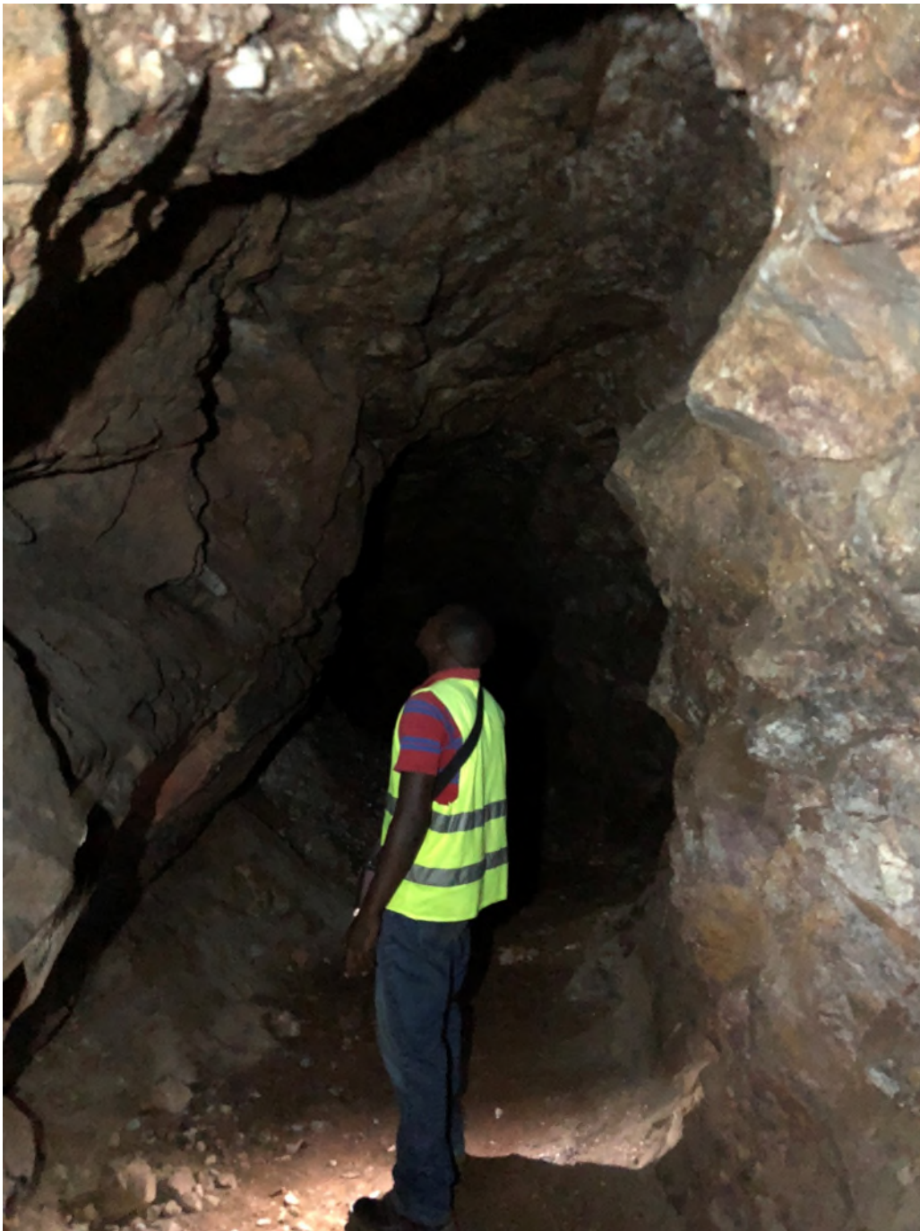
Figure 5 Kikagati Tin Project – Example of a typical larger quartz vein, approximately 2m wide, in one of the many historic workings.
