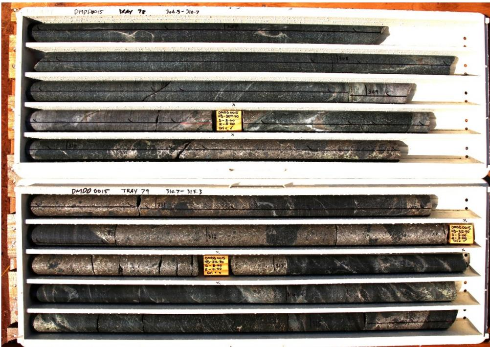
**Figure 4.** Brecciated massive sulphide interval from DMDD0015, core is NQ, from 306.5-315.3m downhole.
