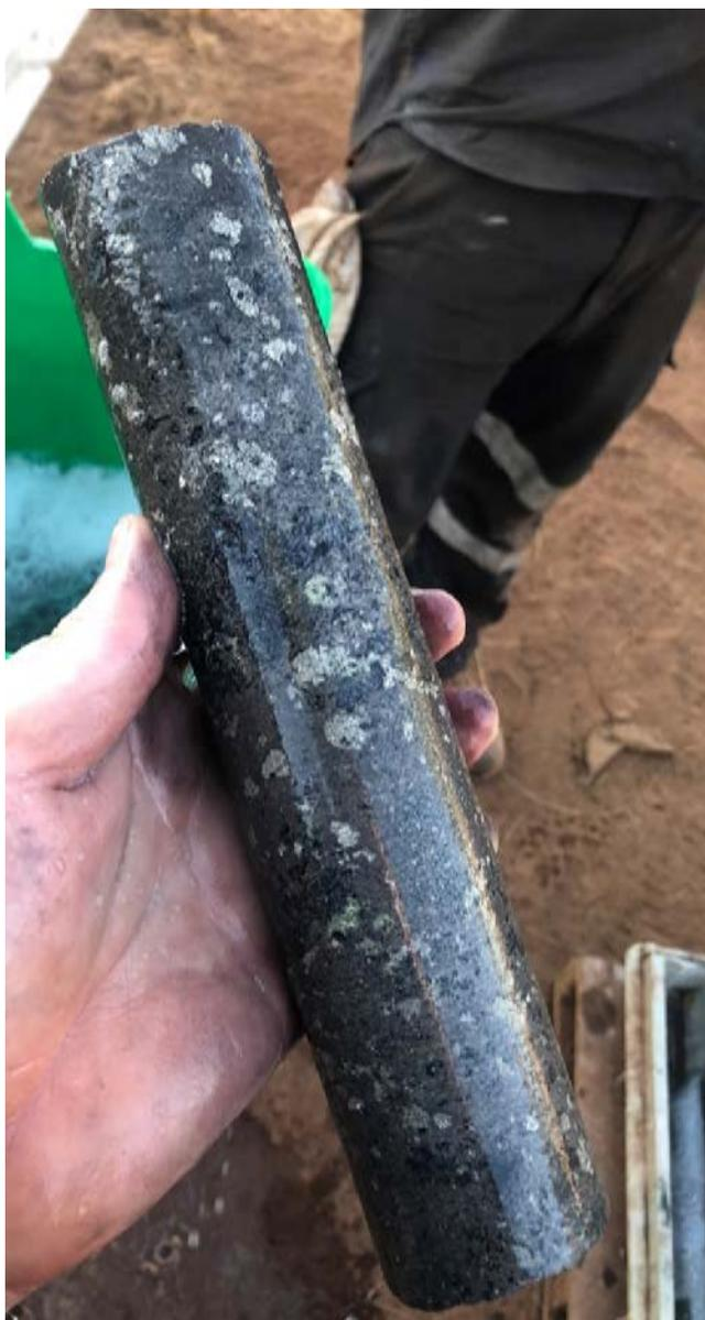
**Figure 5.** Brecciated massive sulphide interval from Zone 1 DMDD0015 312.28 – 312.52m downhole
