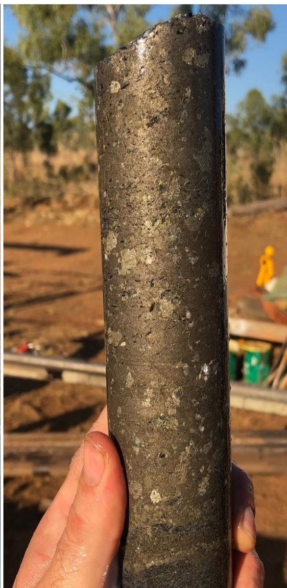
**Figure 4.** Massive sulphide from Zone 3 DMDD0015 342.2 – 342.46m downhole
