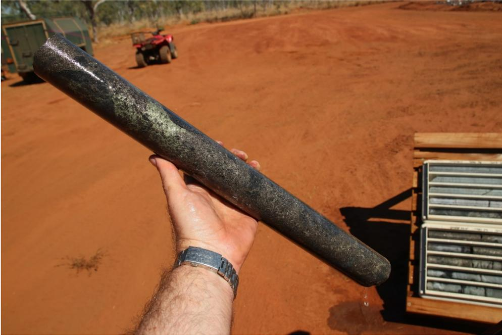
**Figure 3.** Brecciated massive sulphide from DMDD0015 with visible Pentlandite, Chalcopyrite & Pyrrhotite, photograph is of NQ whole core, 310.25-310.72m downhole.
