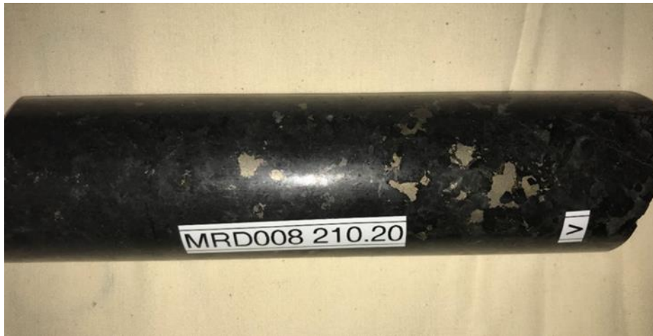
Figure 5. Blebby sulphides hosted in coarse grained pyroxene-olivine meso-cumulate showing visible pentlandite and chalcopyrite.
