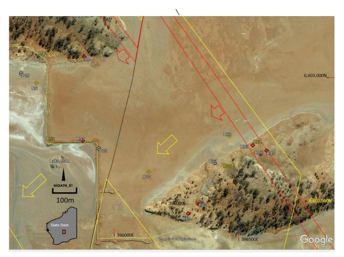
Figure 1: The locations of the successful holes in Phase 3 drilling in June, showing intersection holes (Table 1) in red diamonds and lode trends, steep outlined in red and flat-shallow outlined in yellow. (Image 1.2km by 900m)
