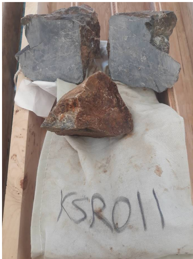
Figure 4. Hydrothermal breccia (KSR011 - 12.15g/t Au, As >10,000ppm, 554ppm Sb).
