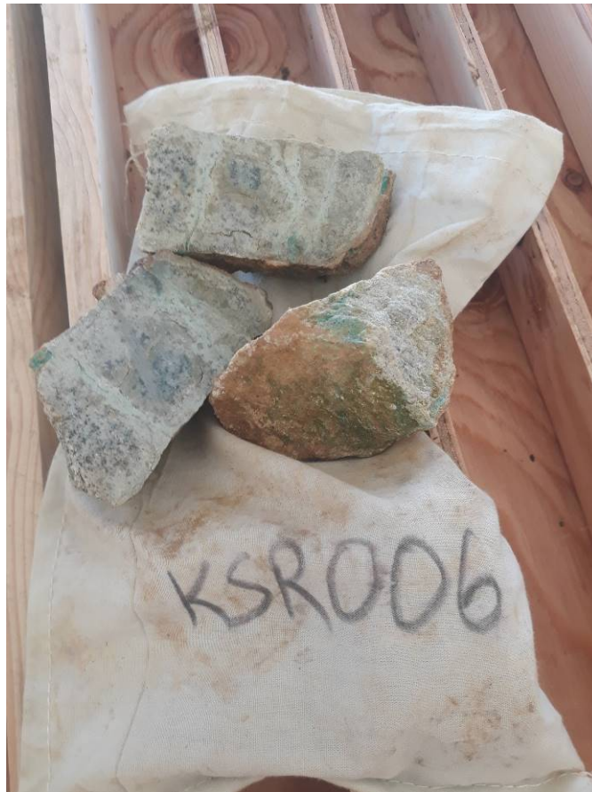
Figure 3. Disseminated sulphides and oxide copper mineralisation within felsic porphyry (KSR006 - 3.35g/t Au, As>10,000ppm, 0.33% Cu).
