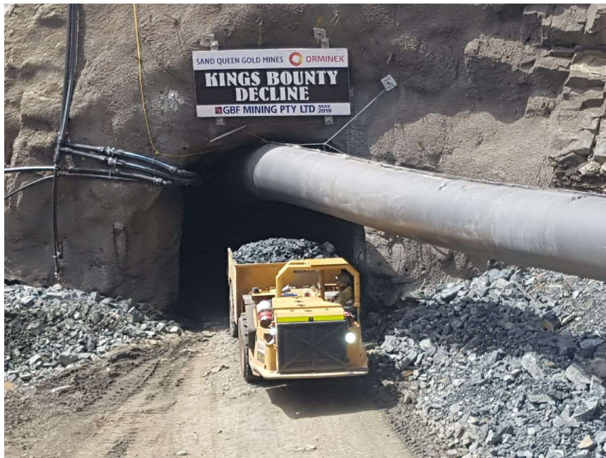
Figure 2 –New low profile 16 tonne truck hauling material
