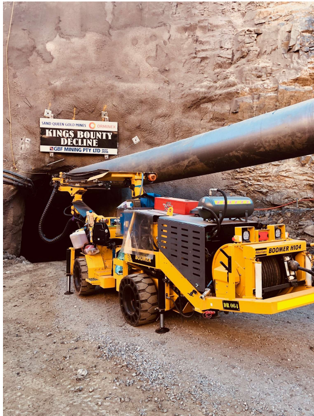
Figure 1 – New Single boom jumbo for ore drive development
