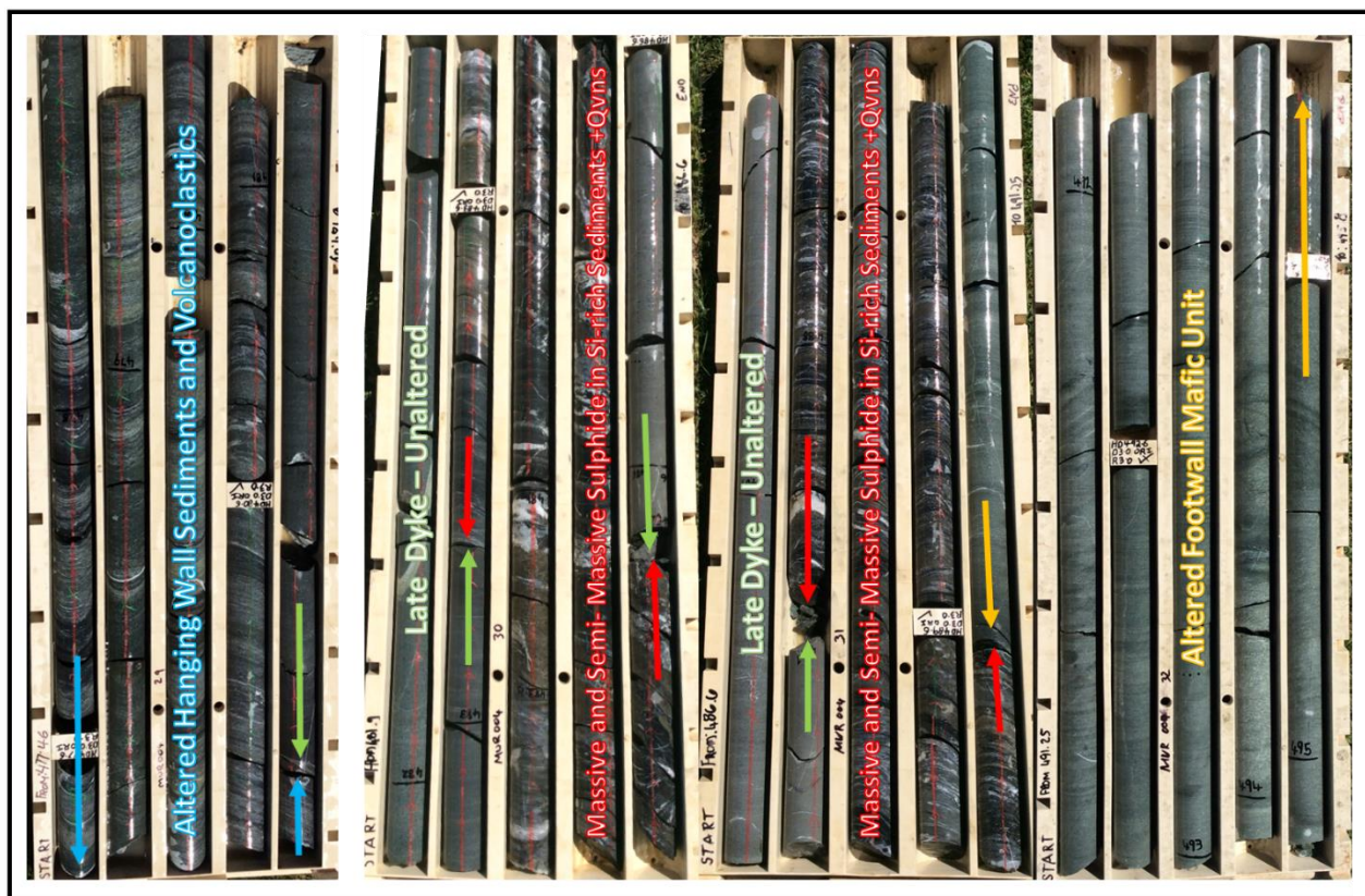
Figure 3: core photos from the zone of interest in MURCDD004 showing a zone of mineralisation surrounded by altered host rocks.
