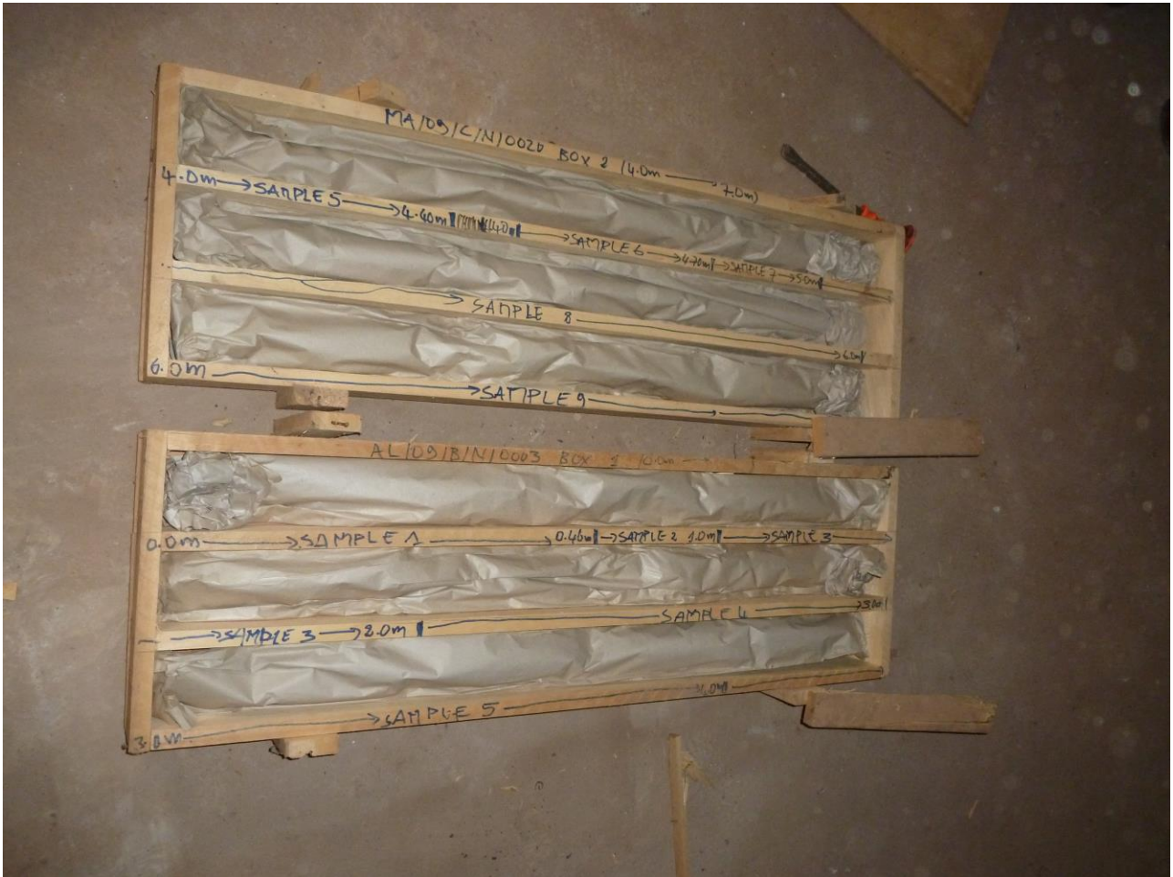
Figure 2: An example of the high quality storage of the drilling core, sealed in wooden boxes and covered
