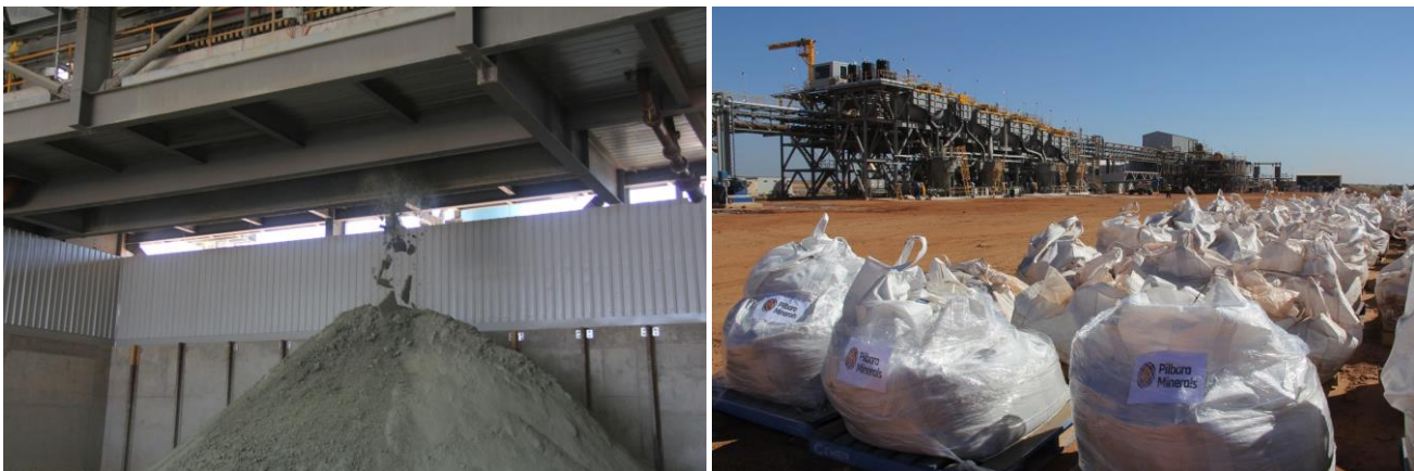
Figure 2: Fines concentrate production from the filter press (top) and tantalite product bags (bottom) ready for delivery.
