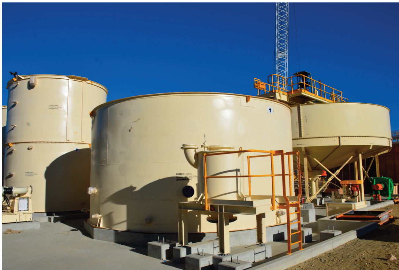
Figure 3: Concentrate storage tanks and thickener (background)
