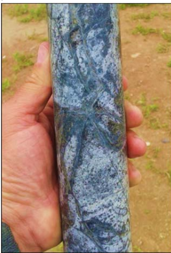
Quartz vein stockwork in hydrothermally brecciated andesite porphyry (hole JS18-002, 446m).
