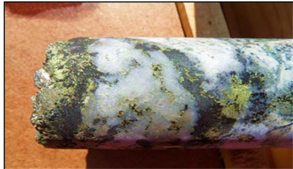
Quartz-tourmaline-pyrite-chalcopyrite vein in strongly altered dacite porphyry (hole JS18-002, 278m).
