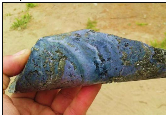
Hydrothermal breccia with "cooling textures" - epithermal veins (hole JS18-002, 451m).
