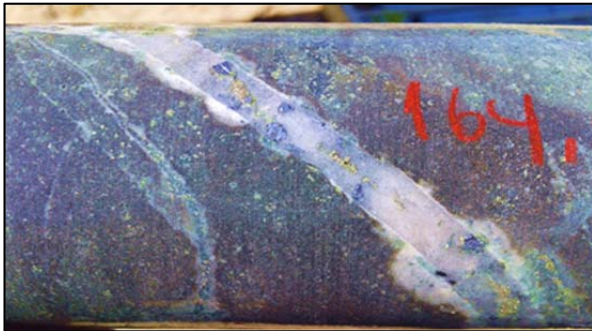
Figure 1 | Quartz-pyrite-chalcopyrite-molybdenite vein (1cm wide) in andesite porphyry (hole JS18-002, 164m).
