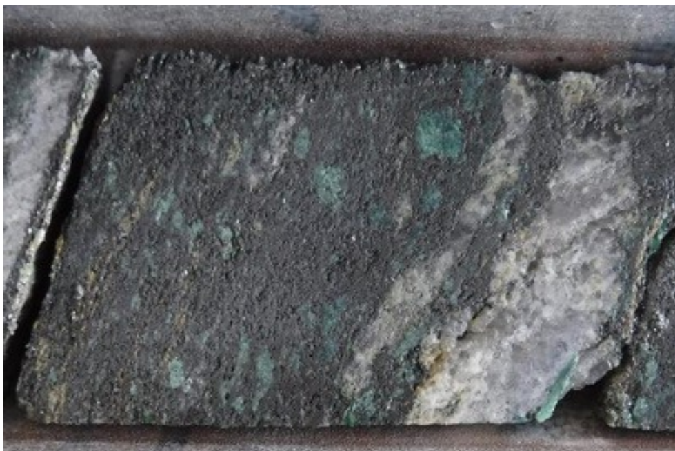
Figure 5. Halved core showing graphitic schist with distinct roscoelite (vanadium-hosting mineral) mineralization
