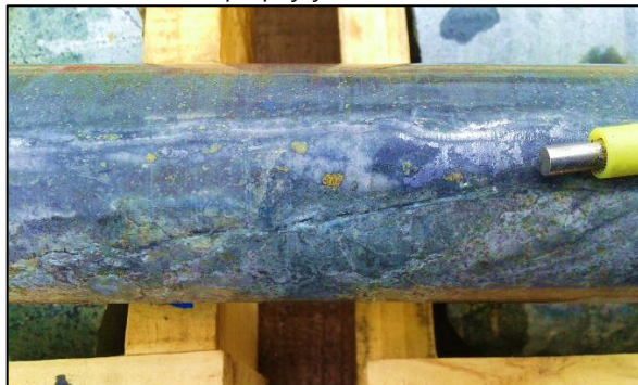
Quartz-sulphide veins and disseminated sulphide in hydrothermal breccia (hole JS18-002, 531m).
