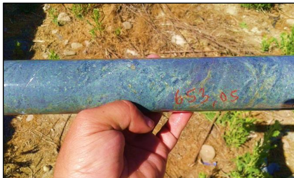
Andesitic porphyry with moderate chlorite and sericite alteration with weak biotite alteration (hole JS18-002, 653m).
