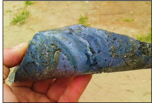
hydrothermal breccia with "cooling textures" - epithermal veins and vugging (hole JS18-002, 451m).
