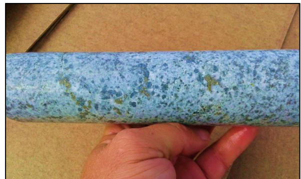
Dacitic porphyry with disseminated sulphide blebs throughout rock matrix (hole JS18-002, 700m)..
