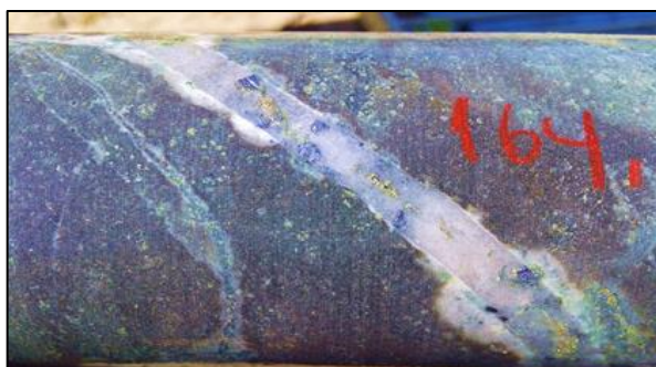
Figure 2 | Quartz-pyrite-chalcopyrite-molybdenite vein (1cm wide) in andesite porphyry (hole JS18-002, 164m).
