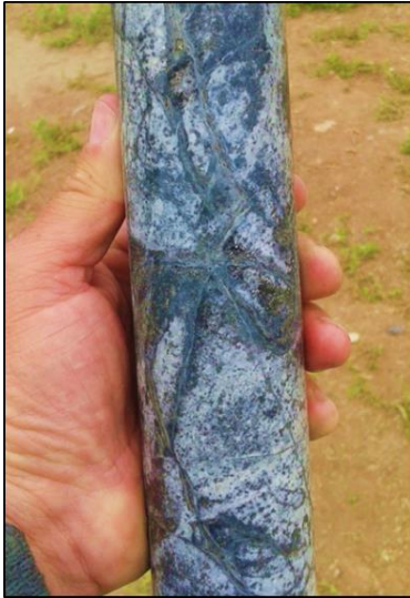
Figure 2 (Cont'd) Quartz vein stockwork in hydrothermally brecciated andesite porphyry (hole JS18-002, 446m).
