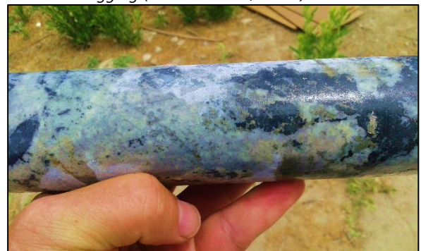
Hydrothermally brecciated porphyry - silica, tourmaline and biotite alteration (hole JS18-002, 618m).
