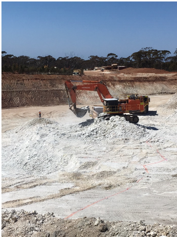
Pioneer geologist (left hand side) communicates with the excavator operator to ensure that waste and KFs are kept separate.
