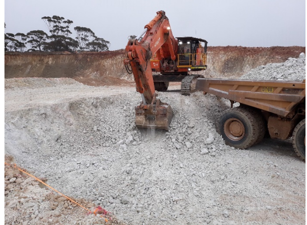
Loading 75 tonnes of K feldspar (KFs) overburden
