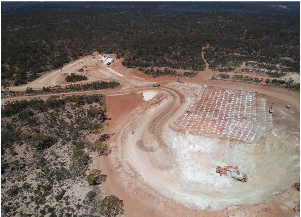
Figure 2: The Sinclair Mine is underway. Excavator and haul truck removing overburden in the foreground. Blast hole rig operating on the right-hand side (a second is parked near the returning haul truck near the centre top).
