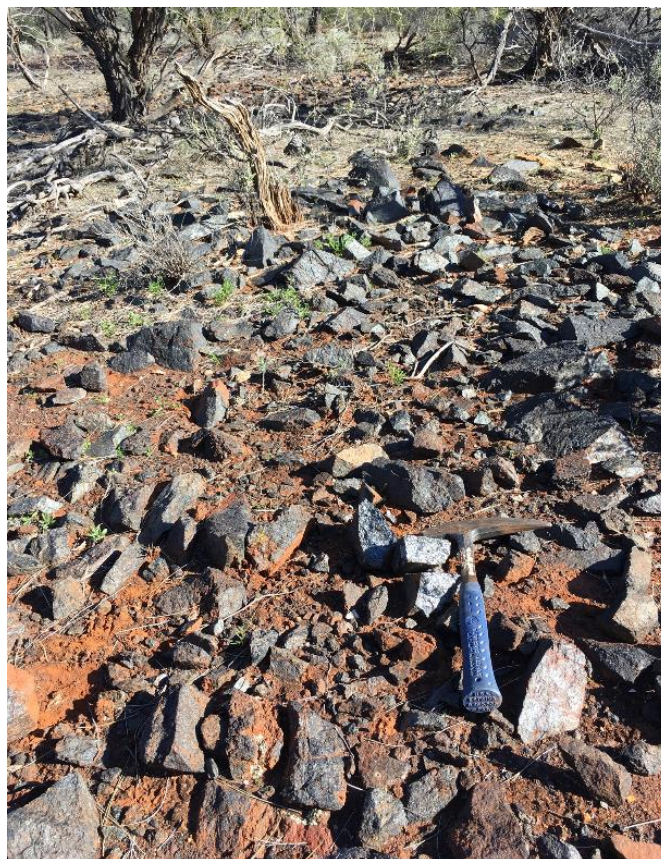
Figure 4 - V205 Rock Chip sampling of Magnetite Outcrops (September quarter 2018) at Watsons Well Prospect
