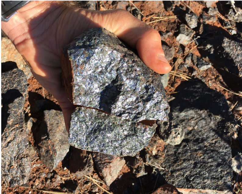
Figure 3 - V205 Rock Chip sampling of Magnetite Outcrops (September quarter 2018) at Watsons Well Prospect
