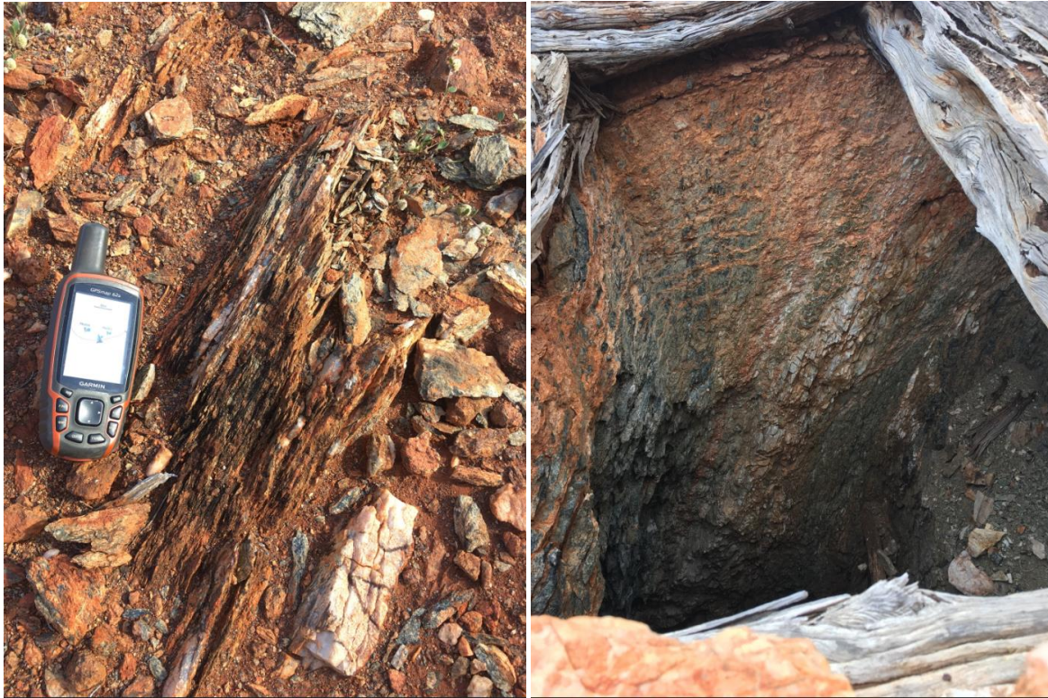
Figure 8 - Surface outcrop (left) and historic Pioneer mine workings (right) of discrete north-south shear zones bearing Au-mineralized quartz veins hosted in massive Leucogabbro rocks
