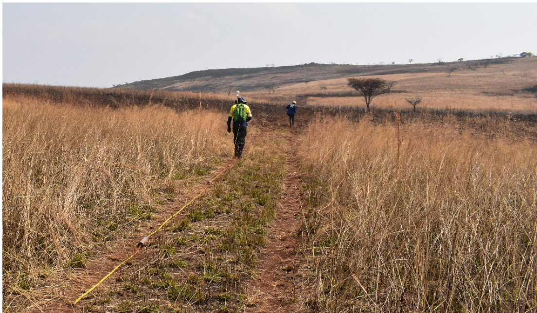
GPR survey in progress over the largely soil covered Longonjo Carbonatite. The GPR tool is the yellow 'snake' trailing behind the surveyor. A DGPS is carried in the backpack
