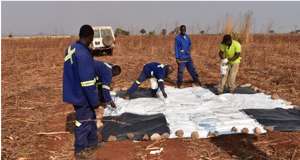
Laying out markers on accurately surveyed Ground Control Points for the satellite topographic land surface survey, August 2018.
