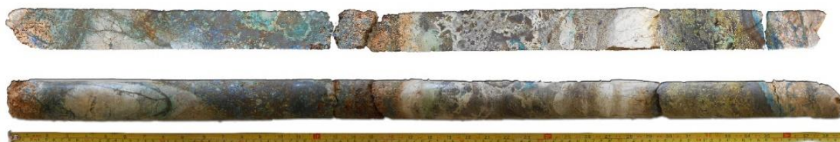
FIGURE 1. Mineralised section of drill core from CMN-3 –136.15-138.10m (1.95m @ 7.72% Cu; 0.11% Co, 0.09% Ni; 0.44% U; 0.24% Zn)
