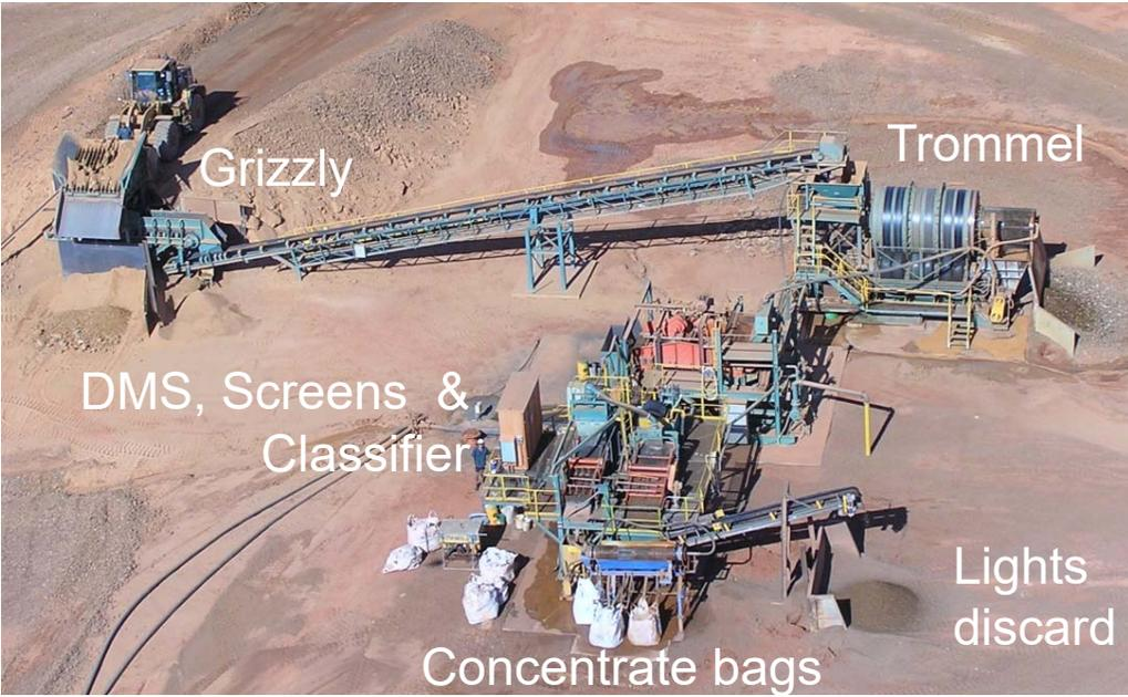
POZ fabricated rotary twin screen unit
