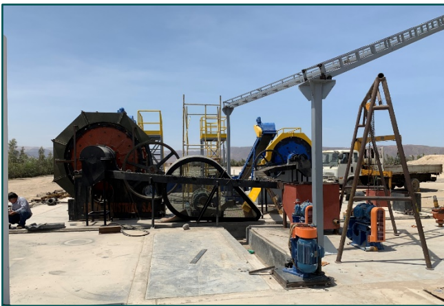
Figure 4 | Grinding Circuit Installed at Vista Plant
