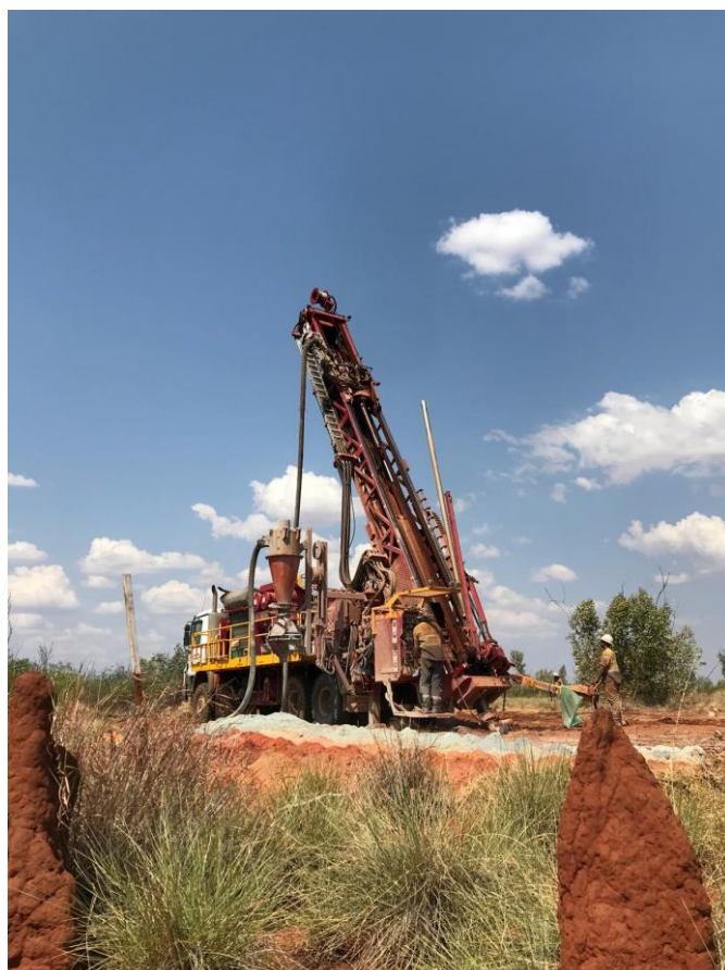
Figure 3. RC Drilling at the Capstan Prospect - October 2018
