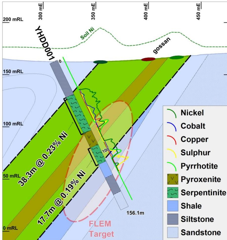
Figure 2: Drill Hole YHDD001 cross section (Young Henry) illustrating significant Ni intersections, down hole geology and traces for various elements.
