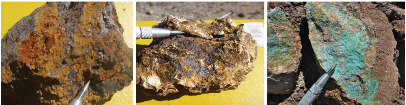
Figure 12 (Above Left): Sample contains 6.52g/t Au and 194g/t Ag; (Above Middle): Gossanous volcanic containing 3.75% Zn, 136g/t Ag and 3.13% Pb. (Above Right): Copper encrusted volcanic containing 0.61% Cu.
