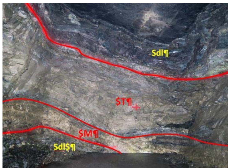
757 ore drive (3.5mW x 3.5mH) @ 6.0% Ni
