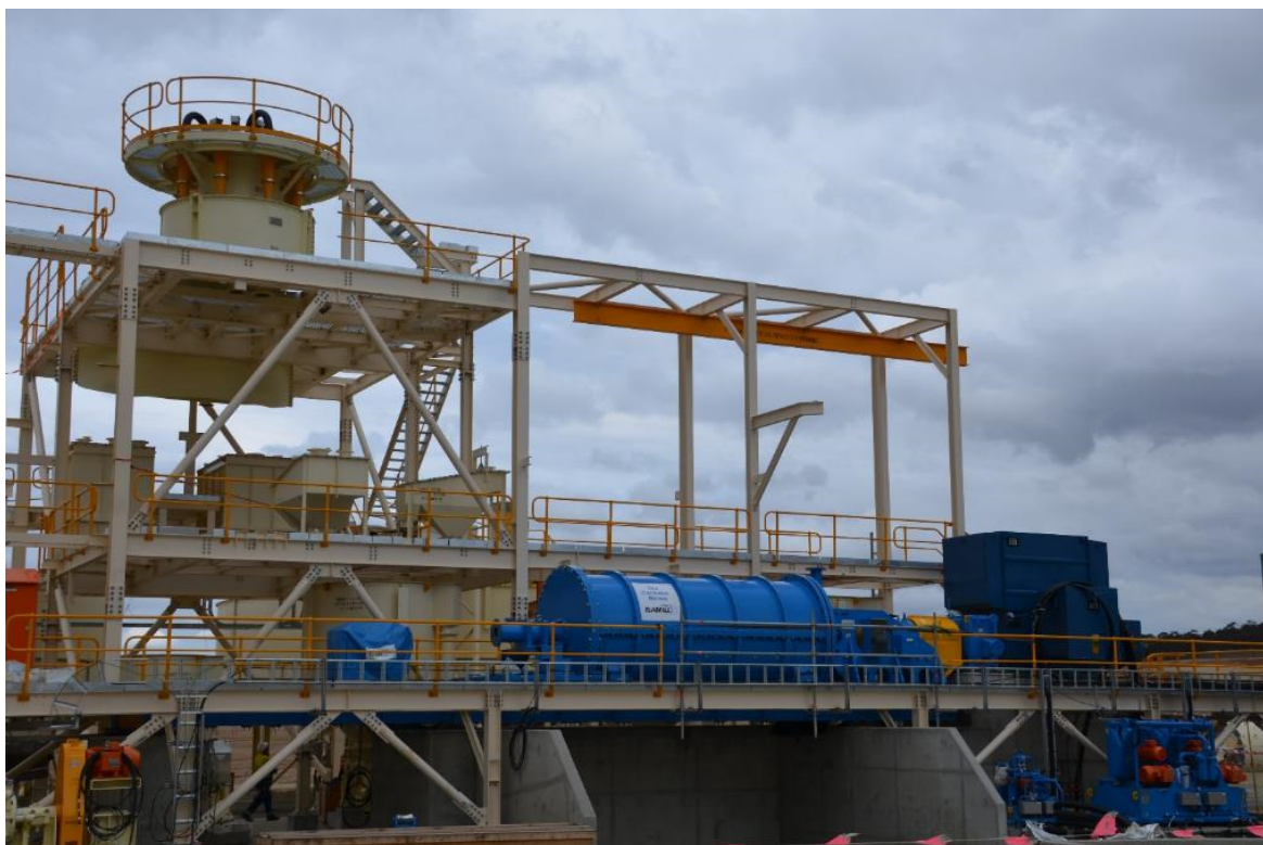
Figure 5: IsaMill™ installed in 4-days in August
