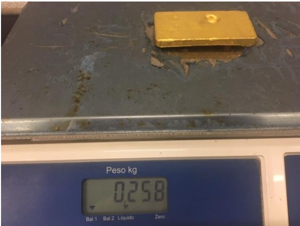
Figure 1. 258 grams of gold recovered from 3 rd party ball mill & CIL processing of 8.94t of Cascavel u/g feed averaging 28.75 g/t
