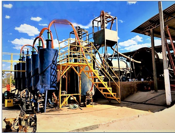
Figure 3. Third party Ball Mill & CIL used for testing Cascavel ore and tailings in August and September
