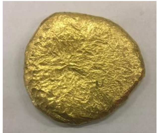
Figure 9. 85.7 grams of gold recovered from 10t of underground ore through our gravity plant.
