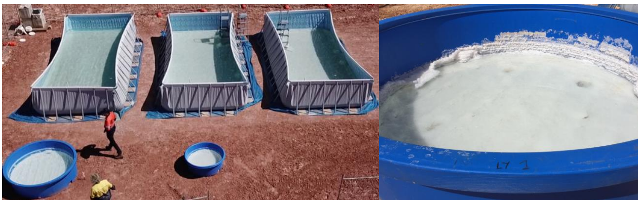
Figure 7: Lake Way – Site Evaporation Trial and first salt forming in Halite Pond
