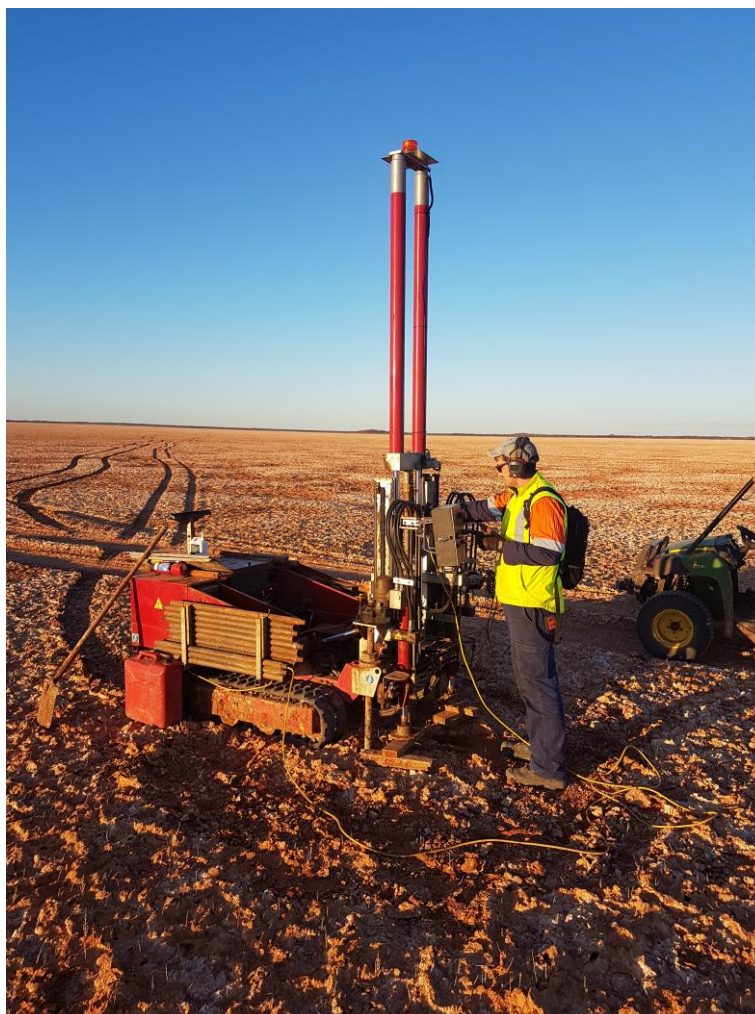
Figure 5: CPT Rig operating at Lake Way
