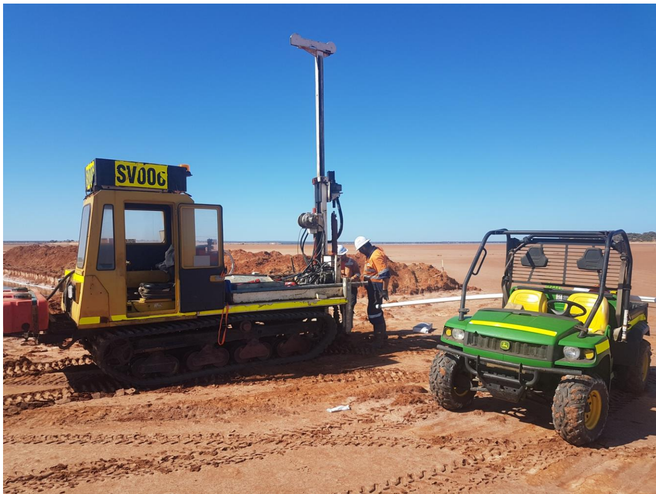
Figure 12: Track Mounted Auger Rig Drilling on Lake Ballard
