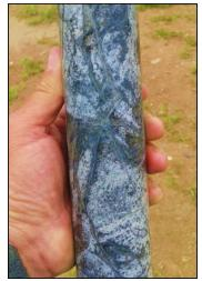
Quartz vein stockwork in hydrothermally brecciated andesite porphyry (hole JS18-002, 446m).
