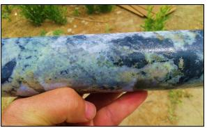
Hydrothermally brecciated porphyry with silica, tourmaline and biotite alteration (hole JS18-002, 618m).
