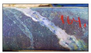
Figure 2 | Quartz-pyrite-chalcopyrite-molybdenite vein (1cm wide) in andesite porphyry (hole JS18-002, 164m).
