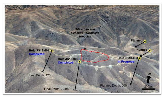
Figure 4 | Relative positions of Manhattan drill holes (completed, in progress and planned) at Joshua shown on north-looking Google image.
