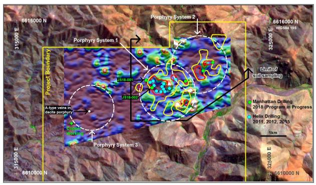
Figure 3 | Imaged aeromagnetic data (analytic signal) showing Helix copper soil anomalies (yellow: +150ppm Cu, red: +500ppm Cu, refer Table 1 for survey details), location of historical drill holes (pale blue dots) and Manhattan drill holes (green dots) and the location of the interpreted three porphyry systems within the Joshua Project Area.
