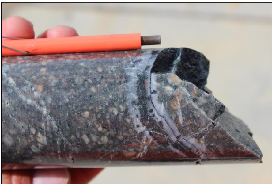
Photo 6. 'B' style vein with magnetite centre at 337.95m in SMD037.
