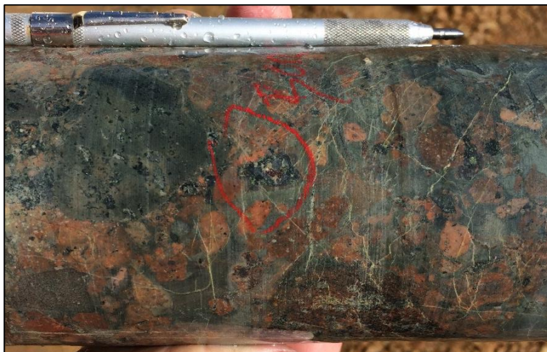
Photo 2. Hydrothermal breccia with bornite in clast at 80m.
