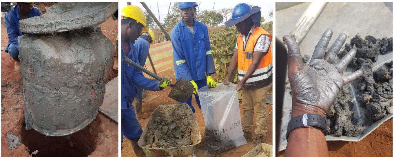
Figure 1. Bulk spiral auger drilling and sampling of the soft, saprolite ore at Malingunde
