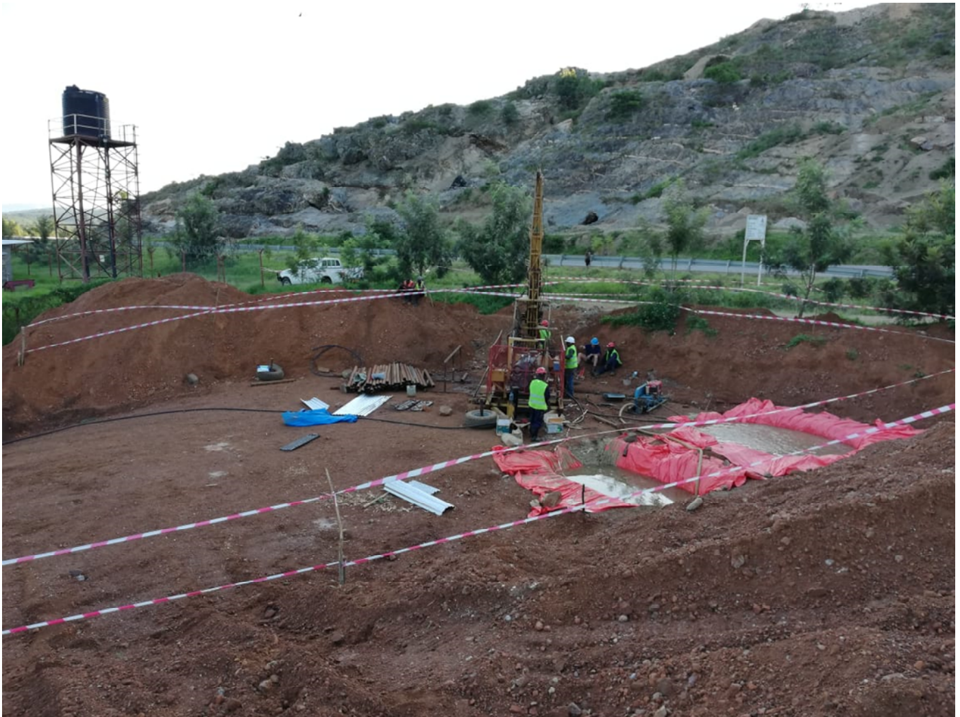
Figure 1 Diamond drilling underway at Kikagati Tin Project, Uganda (Note the quartzite unit dipping towards the rig and quartz veins outcropping along ridge)
