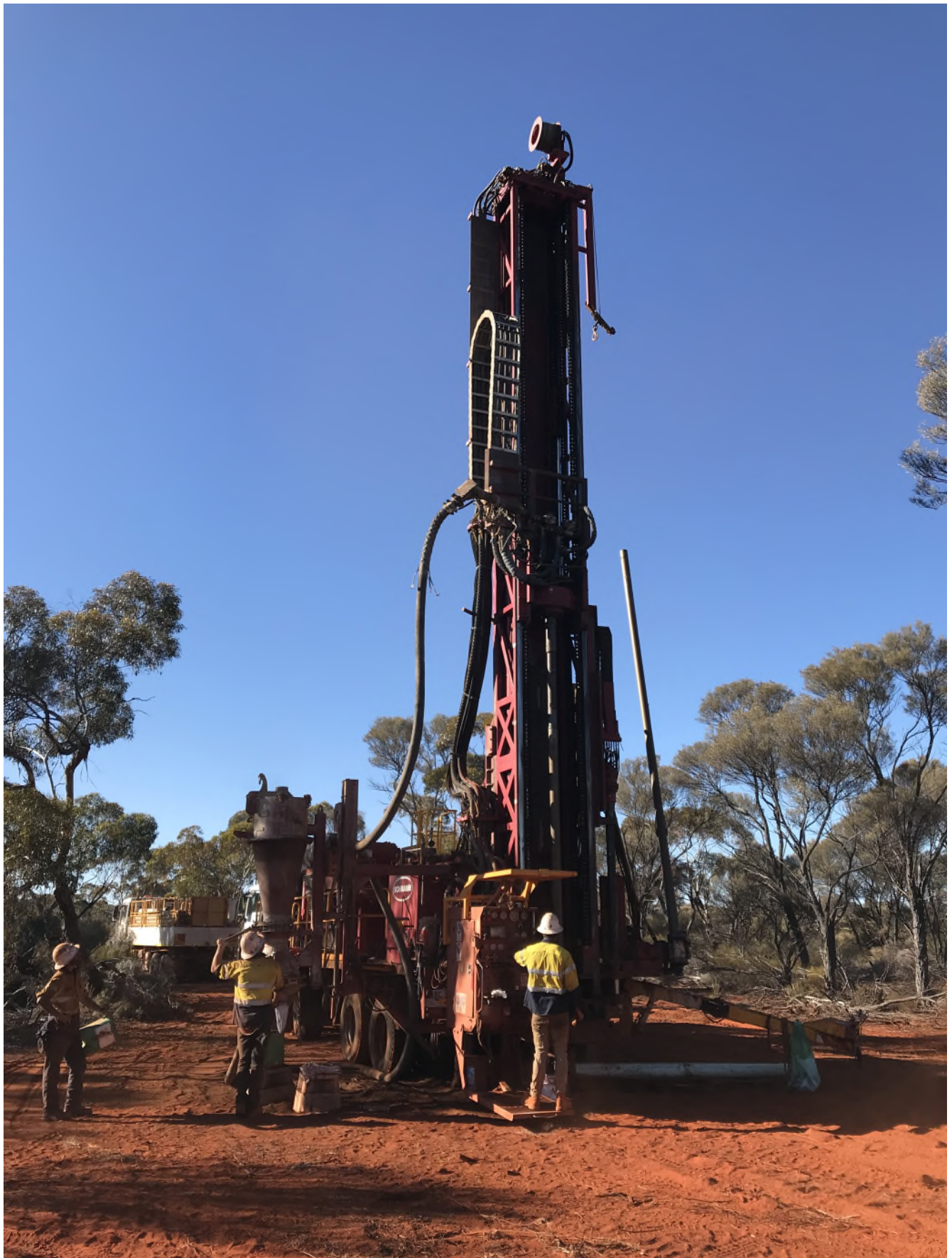
Figure 4 RC drill rig at Grey Dam Nickel - Cobalt Project
