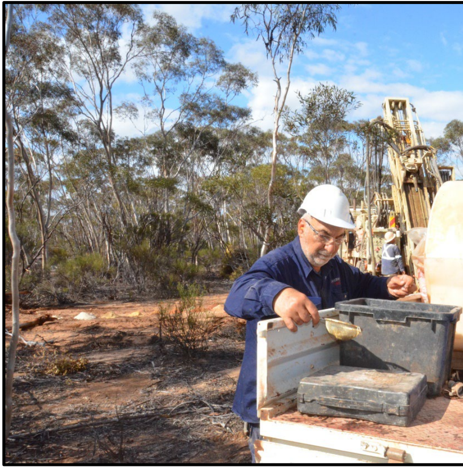
Figure 4: Contract geologist Wilson Gewargis sieving samples and logging end-of-hole geology at Mt Holland East during October 2018
