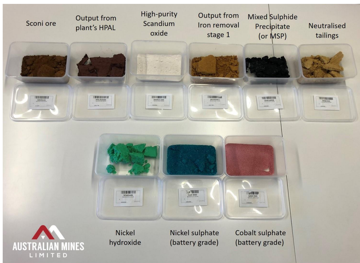
Figure 3: Samples taken from the various stages of Australian Mines' demonstration plant in Perth, Australia. The top row is considered by Australian Mines as the 'front end' of the plant, with the bottom row considered the 'back end' of the plant.
