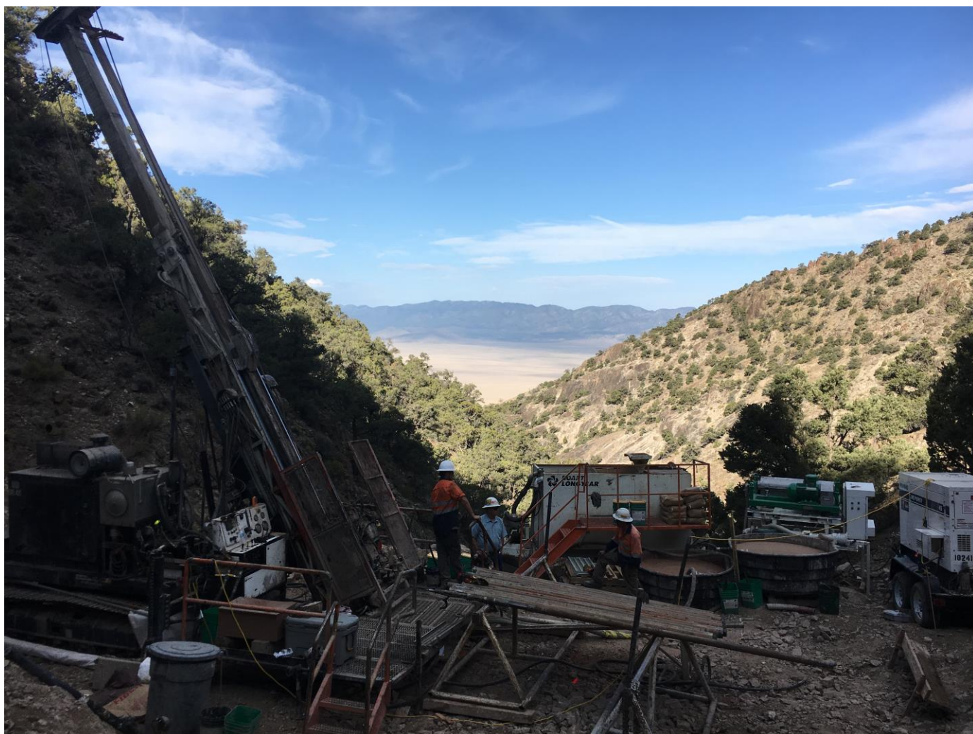
Figure 4: Diamond drill rig at FR18-003.
