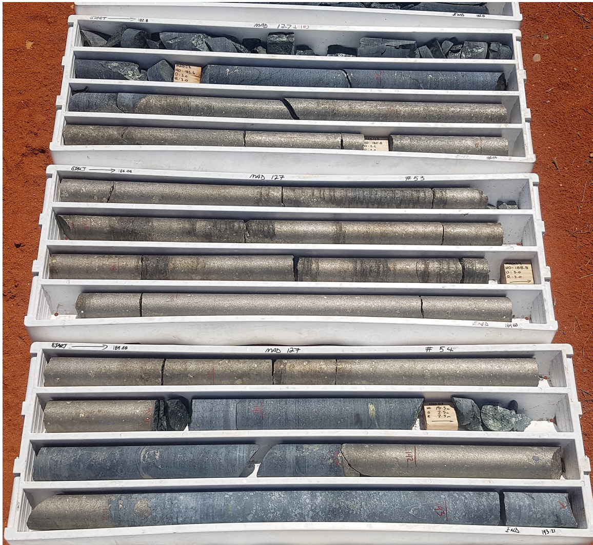
Figure 3 – drill core tray from MAD127 with the thick interval of massive nickel-copper sulphides with average XRF readings of 8.03%Ni and 5.06%Cu.
