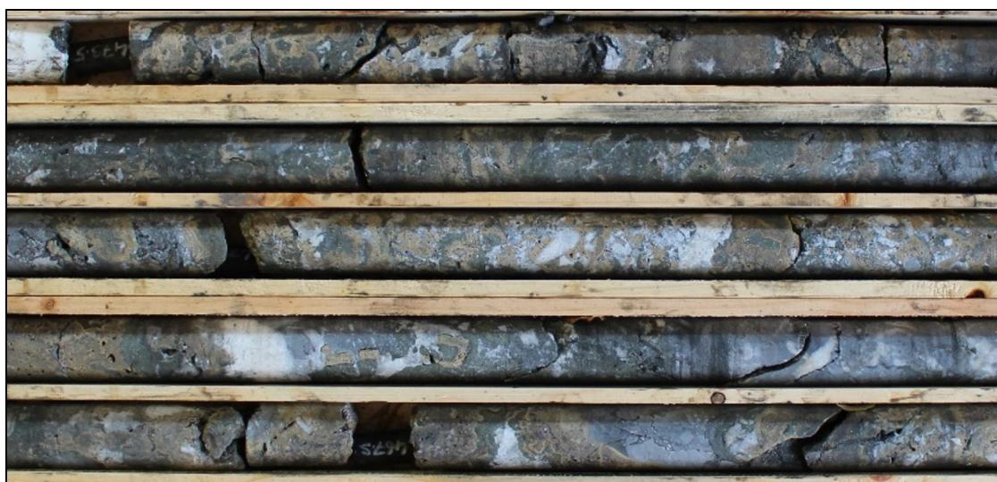
Figure 4: Lengths of high grade massive sulphide mineralisation between 465.0m and 473.6m in Z_4069_027. Tan is sphalerite, greenish is marcasite.
