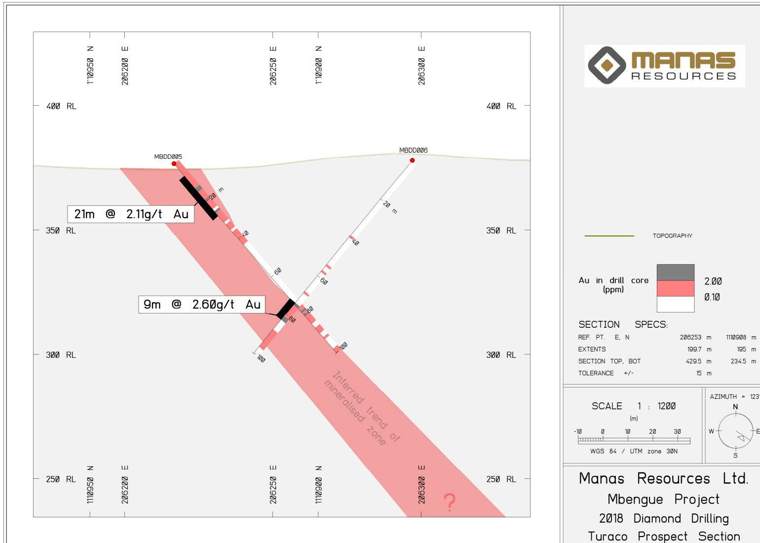
Figure 4: Cross section through the Turaco prospect showing the intercepts in MBDD005 and MBDD006 and interpreted trend of mineralisation.
