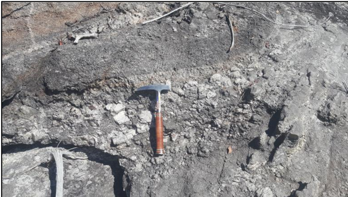
Image 4: PR 4076 lithium bearing pegmatite vein in granite.
