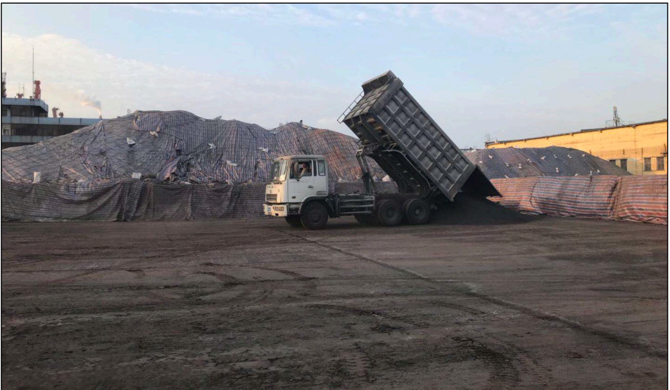
Figure 4: Discharge of New Century concentrate onto a port stockpile prior to transfer to end receiver smelters
