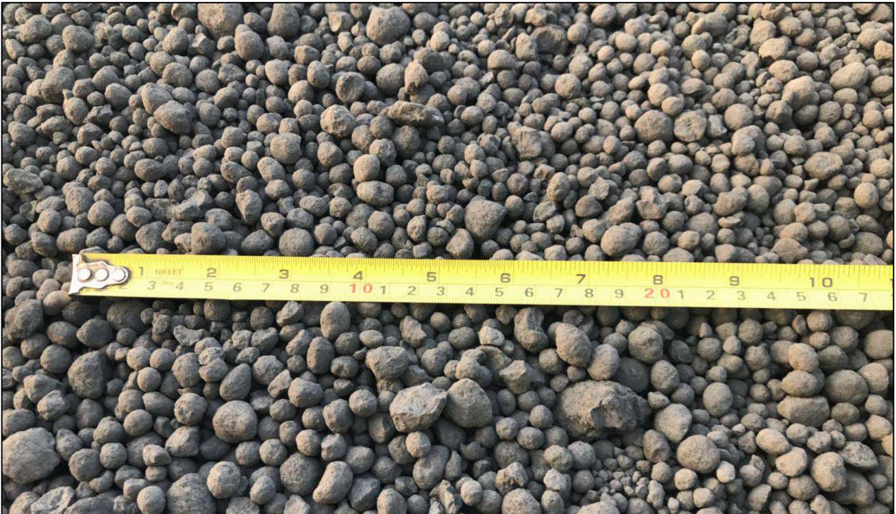
Figure 5: Century zinc concentrate, prilled to contractual specification as per operations over the last 16 years
