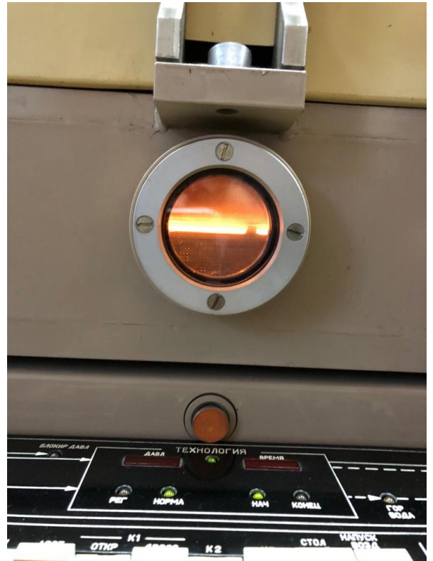
Image 3: Thin film of metal oxides being deposited on substrate for electrode testing
